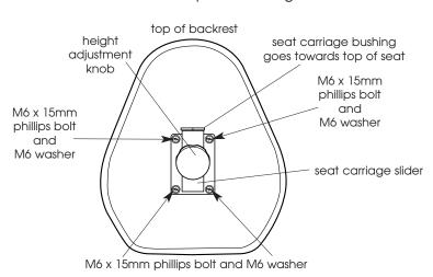
Figure 4b - Install Seat Carriage Slider
